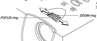
**Note:** The zoom ring allows adjustment of approximately 20% of the maximum screen size. (When the zoom ring is at the center position, an adjustment of approximately ±10% will be possible.)
