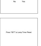
Note: The projector will no longer start when the lamp timer exceeds 1,100 hours. As a result, it will not be possible to reset the lamp timer through timer operations.
