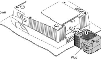
② Tighten the lamp cartridge screw. (Put down the handle of the lamp cartridge.)
